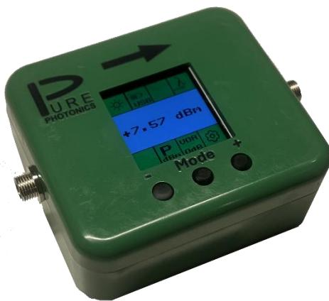
The PPAA1xx in-line power monitor solution provides insight into the power level in your measurement system, without disturbing the optical path and with very low insertion loss. The device continuously monitors the power level in the fiber and when power is detected it automatically activates.
