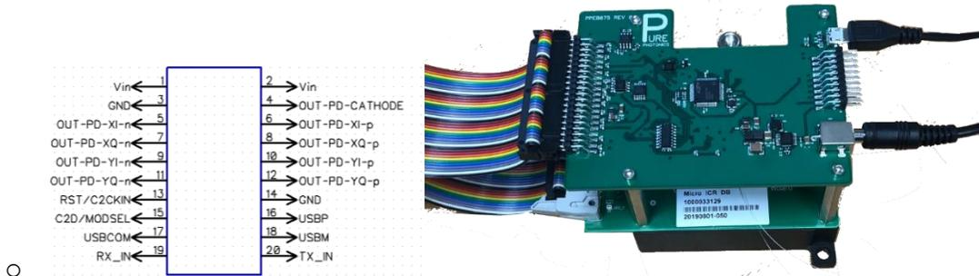
In addition, there is a barrel plug power supply (**make sure that either the pins on the 20 pin connector are connected or this barrel plug. Never connect two power supplies**) with input voltage requirement 10-25V. Typical power consumption is less than 2W.
